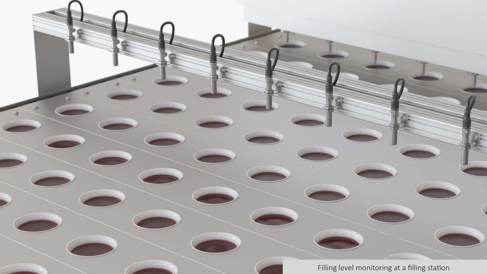
Filling level monitoring at a filling station
