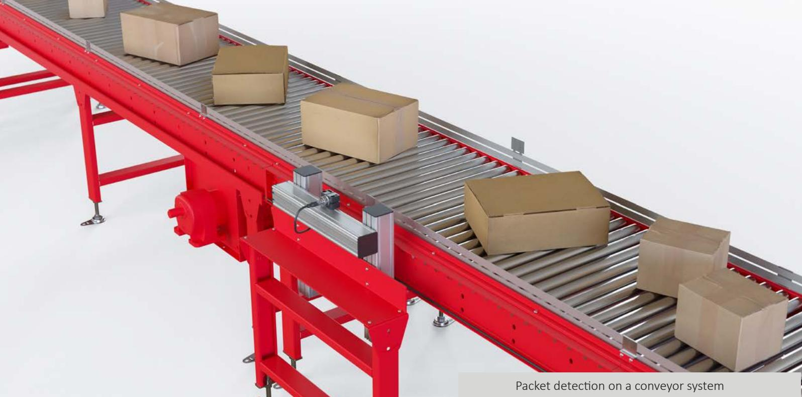
Packet detection on a conveyor system
