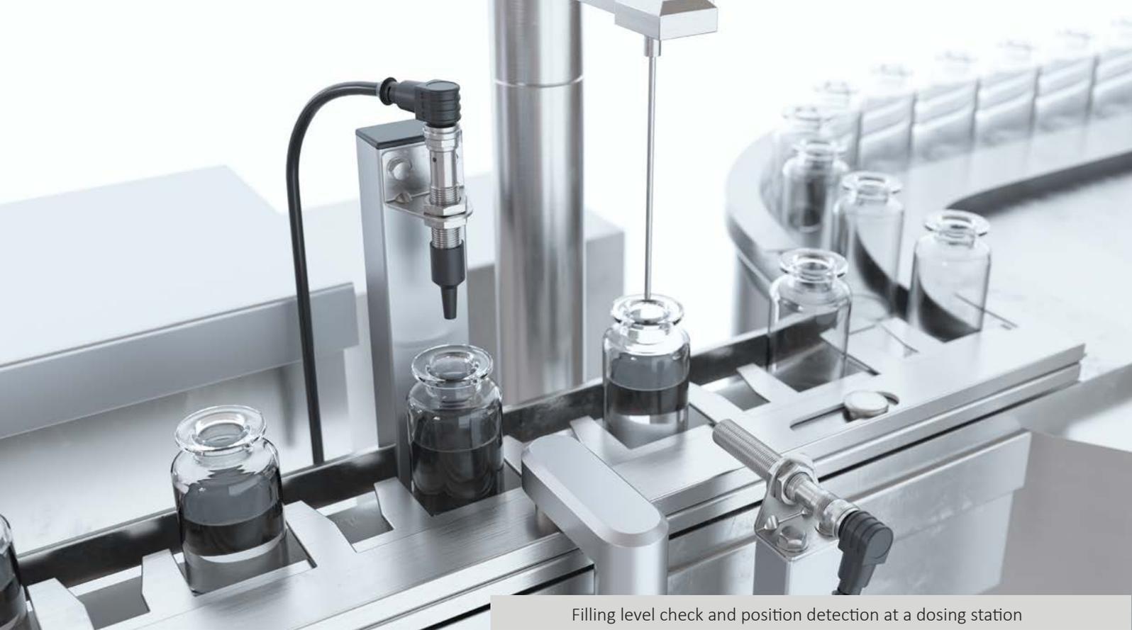
Filling level check and position detection at a dosing station
