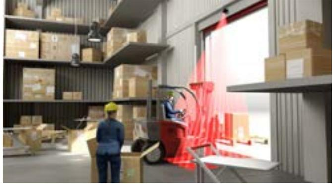
If a vehicle stops in the door area, the presence check of the sensor ensures that the door remains open until the vehicle leaves the detection range of the **RO710900**. Vehicles that merely drive past the gate or persons moving within the detection range of the radar sensor are reliably blanked out.
