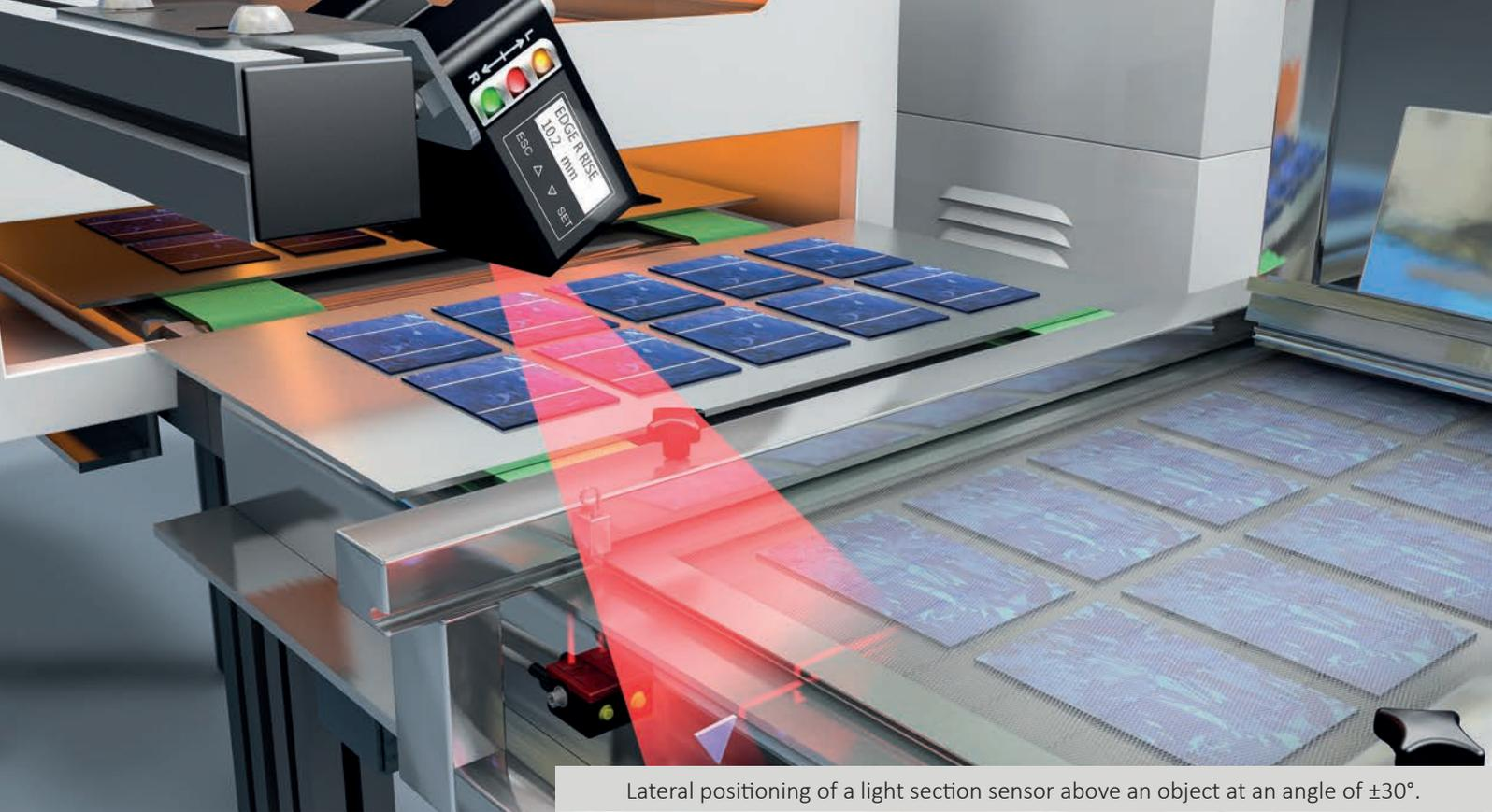
Lateral positioning of a light section sensor above an object at an angle of  $\pm 30^\circ$ .
