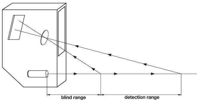
The laser beam is emitted by the transmitter diode and hits the object as a small spot. The sensor's receiver element detects the position of this spot within the "detection range". The sensor basically measures the angle of this position and then calculates the adequate distance. There is a "blind zone" directly in front of the sensor where the objects are not reliably recognized.
