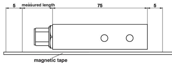
measured length + 35mm + (2\*10mm) = magnetic tape length
