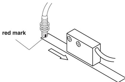
The arrow points to the direction of the linear measurement of the magnetic tape and/or the direction of rotation of the magnetic ring (signal A before B). Please observe the red marking when positioning the sensors for **MW08**! An indication for positioning the **MW10** is the cable outlet.
