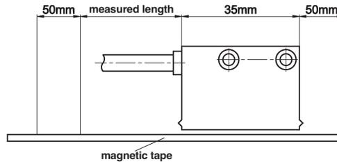
**measured length + 35mm + (2\*50mm) = magnetic tape length**
