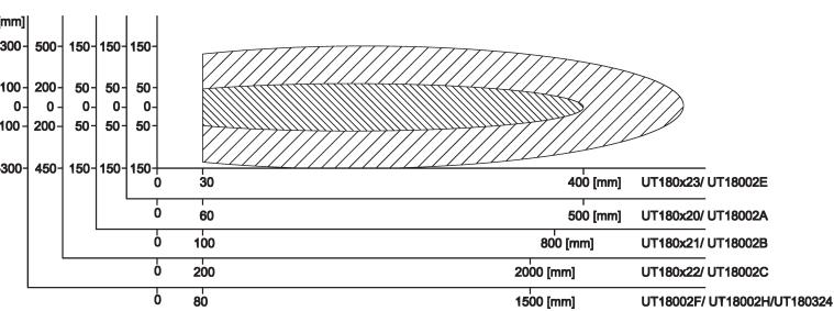
▀ definite detection of an object of 100x100mm   ▲ possible detection of a large object
