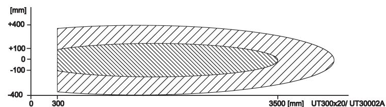
definite detection of an object of 100x100mm
