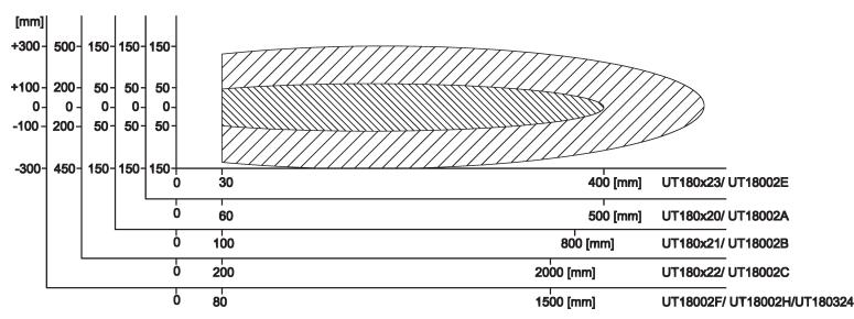
definite detection of an object of 100x100mm
