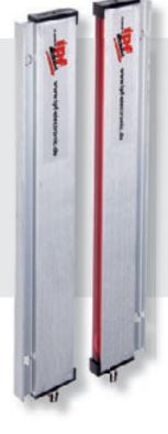
The OYL2 fully automatic light barriers round off the comprehensive range of solutions for presence and movement monitoring. With their integrated electronics, a flat design of just 9mm, operating ranges of 5m (optional: 10m) and lengths of 240mm to 3030mm, these light barriers are ideal
