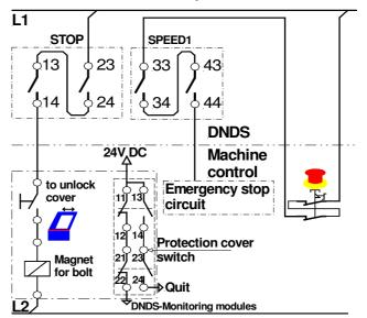
If it necessary the stop contacts can be serial, the speed contact can be parallel and contrary.
