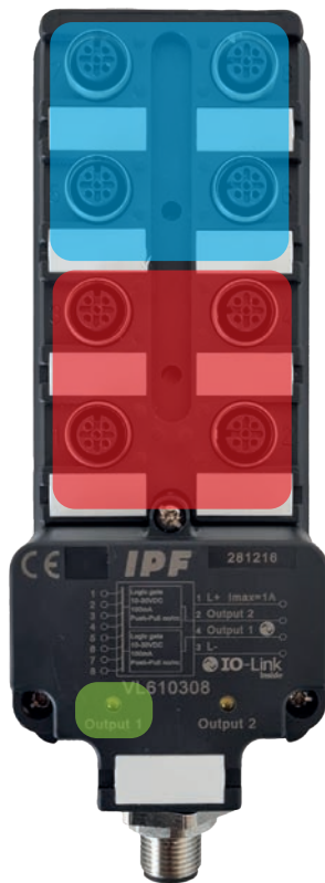
(Figure 1 with color coding: 8-fold logic module with AND link at output 1 for inputs 1 to 4. OR link for inputs 5 to 8.)
