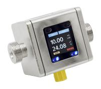
If an electrically conductive liquid moves across a magnetic field, a voltage is generated perpendicular to this magnetic field that is dependent on the flow velocity. This voltage is measured by electrodes located in the wall of the measuring tube. Microcontrollers evaluate this voltage, calculate the flow rate and show it on the display. An analog signal and a transistor switching output are available for further processing.
