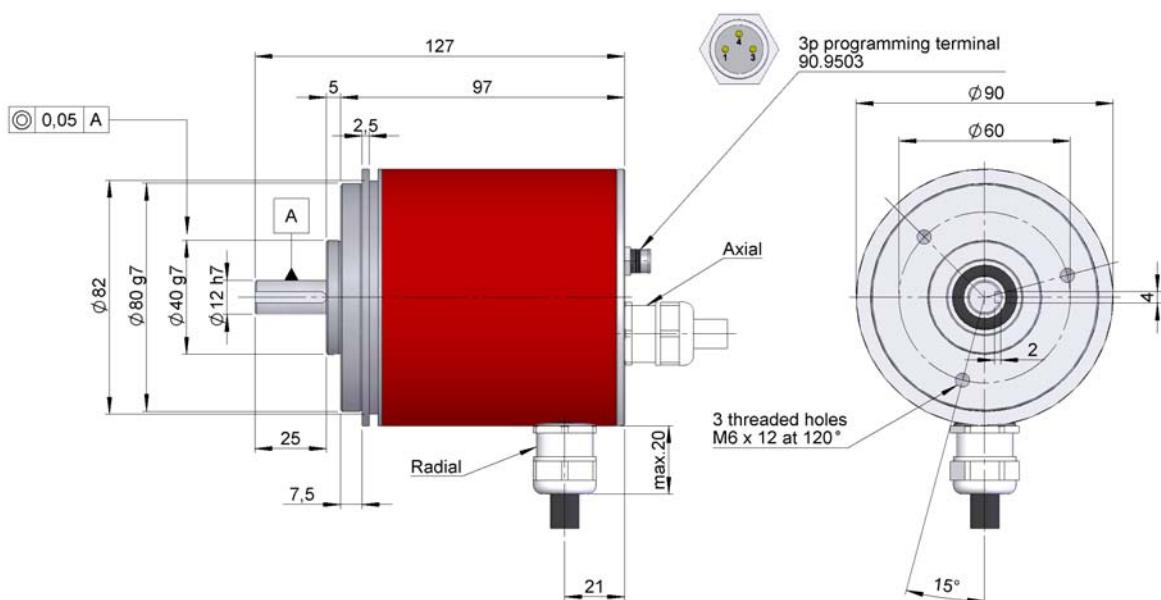
Previous mounting and installation of the encoder is recommended to read the section "TECHNICAL CONSIDERATIONS".
